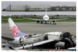
went up in flames soon after landing at Naha Airport the previous day.TOSHIYUKI TSUNENARI/ THE ASAHI SHIMBUN They suspect the fuel leaked from the pylon that connects the main wing and the right engine, according to investigation officials.
